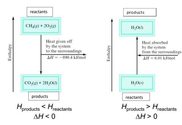
$\Delta H = H_p - H_R =$  negative So , it is exothermic reaction System gives off heat
